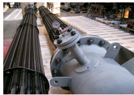
Tank heating coils
