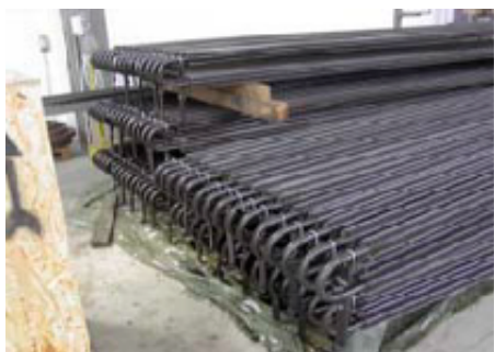
Tank heating coils
