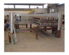
Carbon Steel – Stainless Steel and special Alloys (Nickel, Cupronickel, Duplex, Super Duplex) materials welded longitudinally and helical finned pipes
